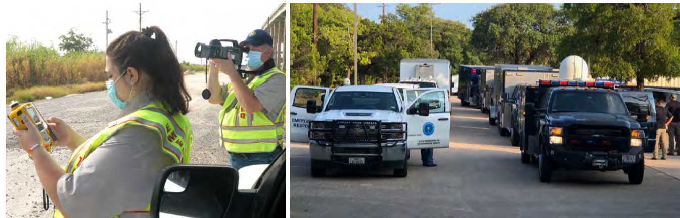
(Left) Agency staff use handheld monitoring equipment in use in the aftermath of Hurricane Laura. On the left, a MultiRAE reports data directly from the field. On the right, an Optical Gas Imaging Camera (OGIC) detects gases and emissions quickly, accurately, and safely. (Right) TCEQ and other emergency response personnel prepare to depart for the Texas coast to assist in the wake of Hurricane Laura.
