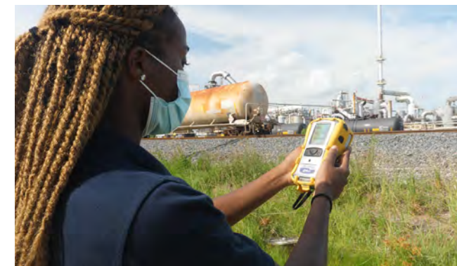
TCEQ staffer using a MultiRAE after Hurricane Laura. These handheld monitors provide instantaneous readings for various compounds when present in the air.
